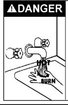
Water temperature over 125°F (52°C) can cause severe burns instantly resulting in severe injury or death.
